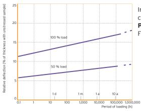
Increase in deformation under consistent loading
